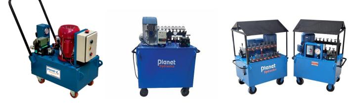
P - Power Pack Unit, H - Hand Lever Operated, S - Single pump, D - Double Pump, PB - Push Button Operated 2 - Hp + Three Phase L - Liter
